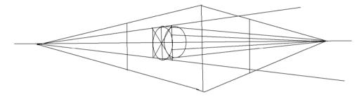
On removing all the construction lines, we can see in the drawing below that the wheel now looks attached to the building and not floating separately from it and this is purely because the same vanishing point of being used for the wheel and for the building.
