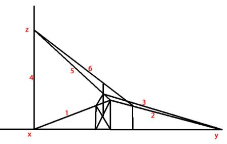
the roof (z). Now a line is taken from the far corner of the building up to this vanishing point (6), which gives us the angle of the distant end of the roof. We can see that the apex of the roof is not parallel to the gutter line, and the near and distant ends of the roof disappear to the vanishing point that belongs to the roof and are different and must not be drawn parallel. I see students trying to make these parallel and they look so wrong.
