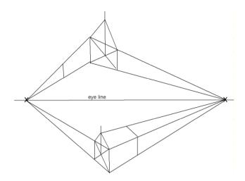
How do we get the apex and the distance roofline? If we look at the figure below we can see from the vanishing point that is relative to the gable end (x), a vertical line is drawn (4). Then the near roofline is taken up to intersect that vertical (5) this gives us a vanishing point for
