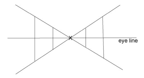
In this picture our eyes were half way up the nearest building. If we were to lay on the ground making the ground our eyeline, we can see that all the lines go down to the vanishing point, and none are going up to it.
