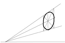
we are looking at the circle with our eye line through the centre but it may be that the circle is above or below the eye line. If the circle is above the eye line we must draw the box above the eye line, followed by the diagonals to give is the centre of
