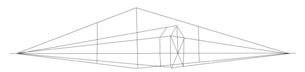
Now removing all the construction lines we can see that the porch looks attached to the building. So it is important in perspective that we consider parallel faces, all faces that are in line or parallel must go to the same vanishing point.
